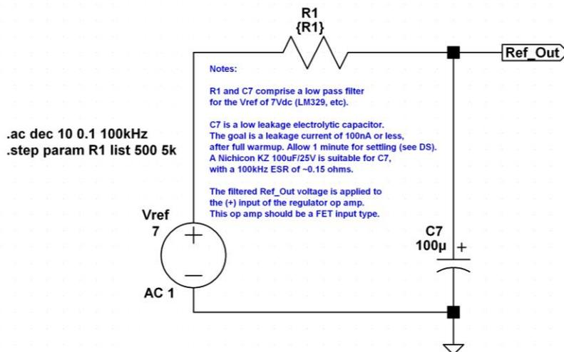
corresponds to 100nA, or equivalent to 0.1μA of current. Nichicon type UFG samples were almost as low in tested DC leakage.
