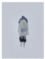
In doing this final step, first use squeeze some silicone compound within the tubing, before applying it over and around the GLED431circuit. This step surrounds and isolates D1/Q1 within the silicon, as well as holds the tubing in place, once the silicon has set up.
