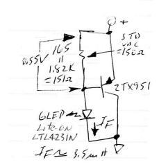
This GLED431 circuit is very simple, and works as a 2.5V shunt reference with ultra low noise.
