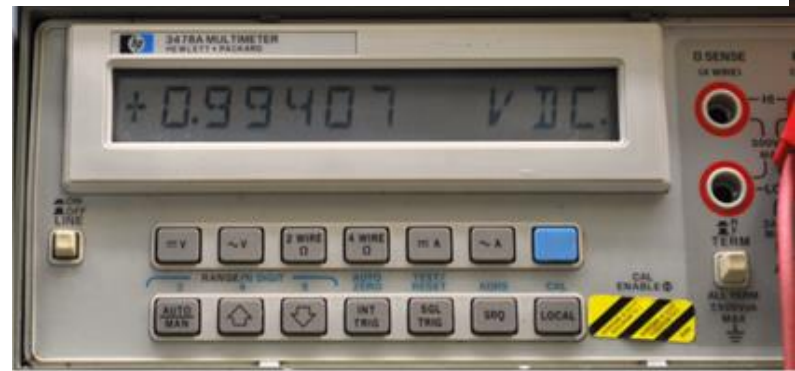
Picture 2.3 An Untrimmed Output from the Picture 2.2 Setup with R_5 = 0
