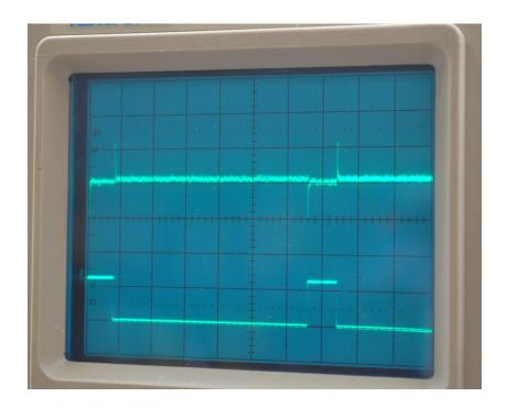
100mA (lower trace). The pulse risetime is controlled at ~10 $\mu$ s, consistent with audio bandwidths. Artifacts are the residual wideband baseline noise, mostly the AD825 op amp input noise. There are also narrow transient switching spikes. The spikes appear in all the readings taken, but are considered benign, as real audio signals likely won't have 10 $\mu$ s risetimes. See more on this under the **Spikes:** section.
